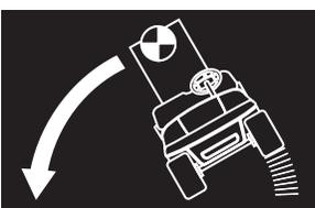
**LOAD WITH HIGH CENTER OF GRAVITY COULD RESULT IN TIP OVER**
