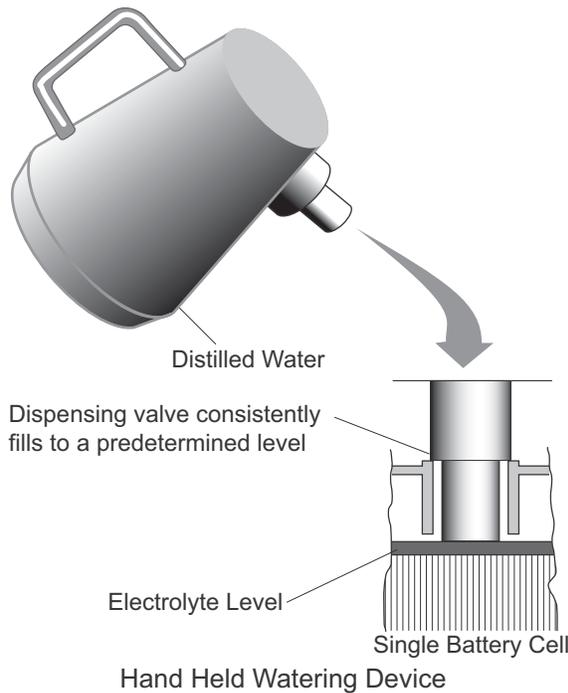
Watering gun similar to the type included in the E-Z-GO Battery Maintenance Kit
