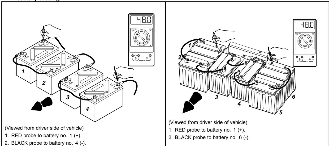
**Figure 13-6 Battery Voltage Test – 4 x 12 Volt Battery Configuration**
