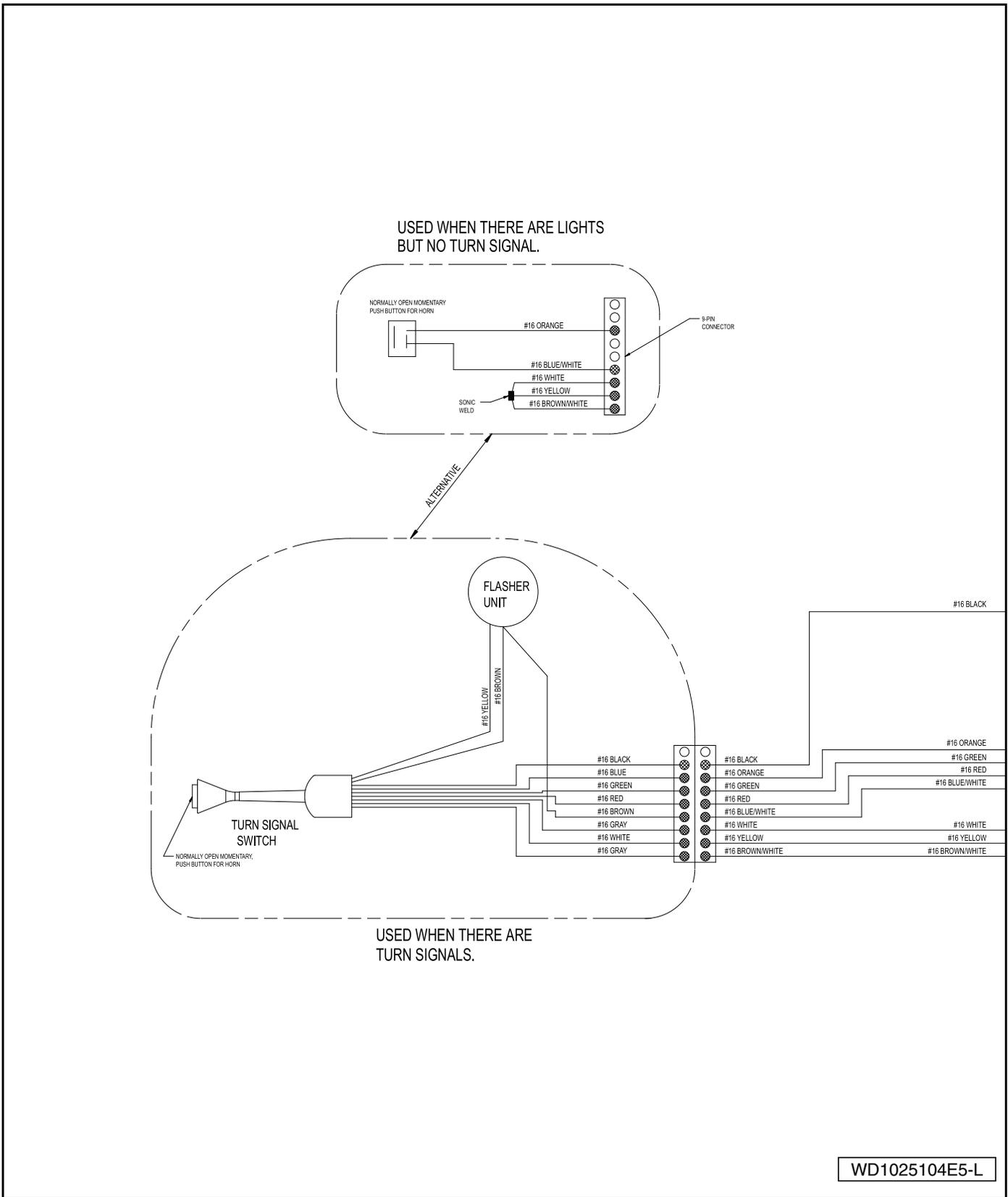
Figure 12-3 Precedent Electric Vehicle Accessory Wiring Diagram
