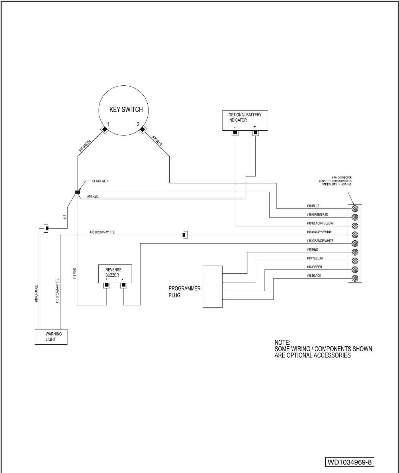
Figure 11-5 Precedent Electric Vehicle Instrument Panel Wiring Diagram
