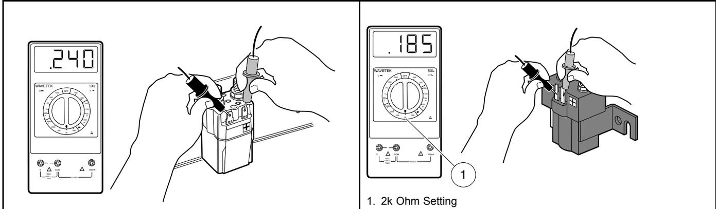
Figure 12-9 Activating Coil Test – Factory-installed Solenoid
