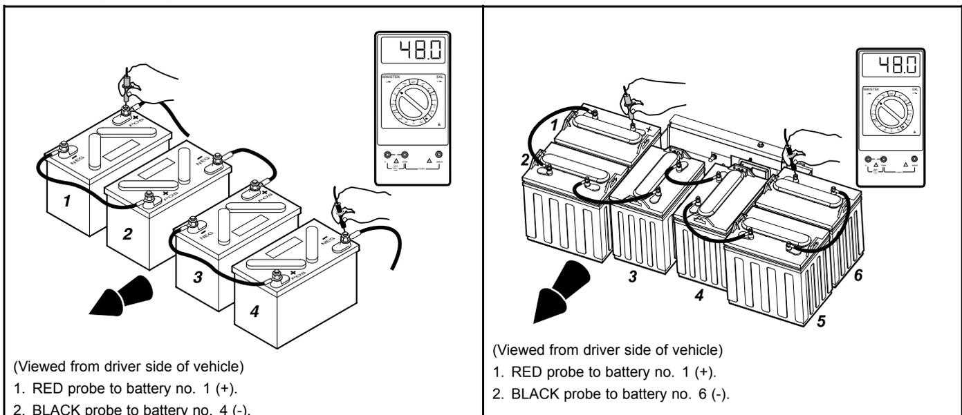
**Figure 14-6 Battery Voltage Test – Style B Battery Configuration**
