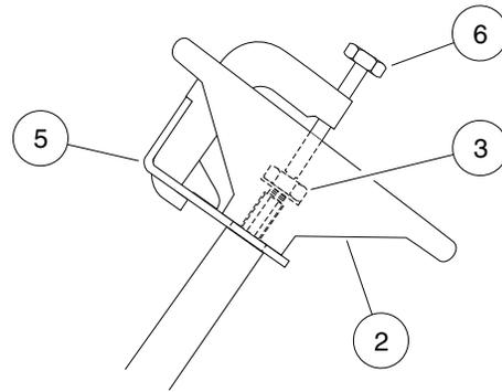
Figure 7-2 Steering Wheel Puller
