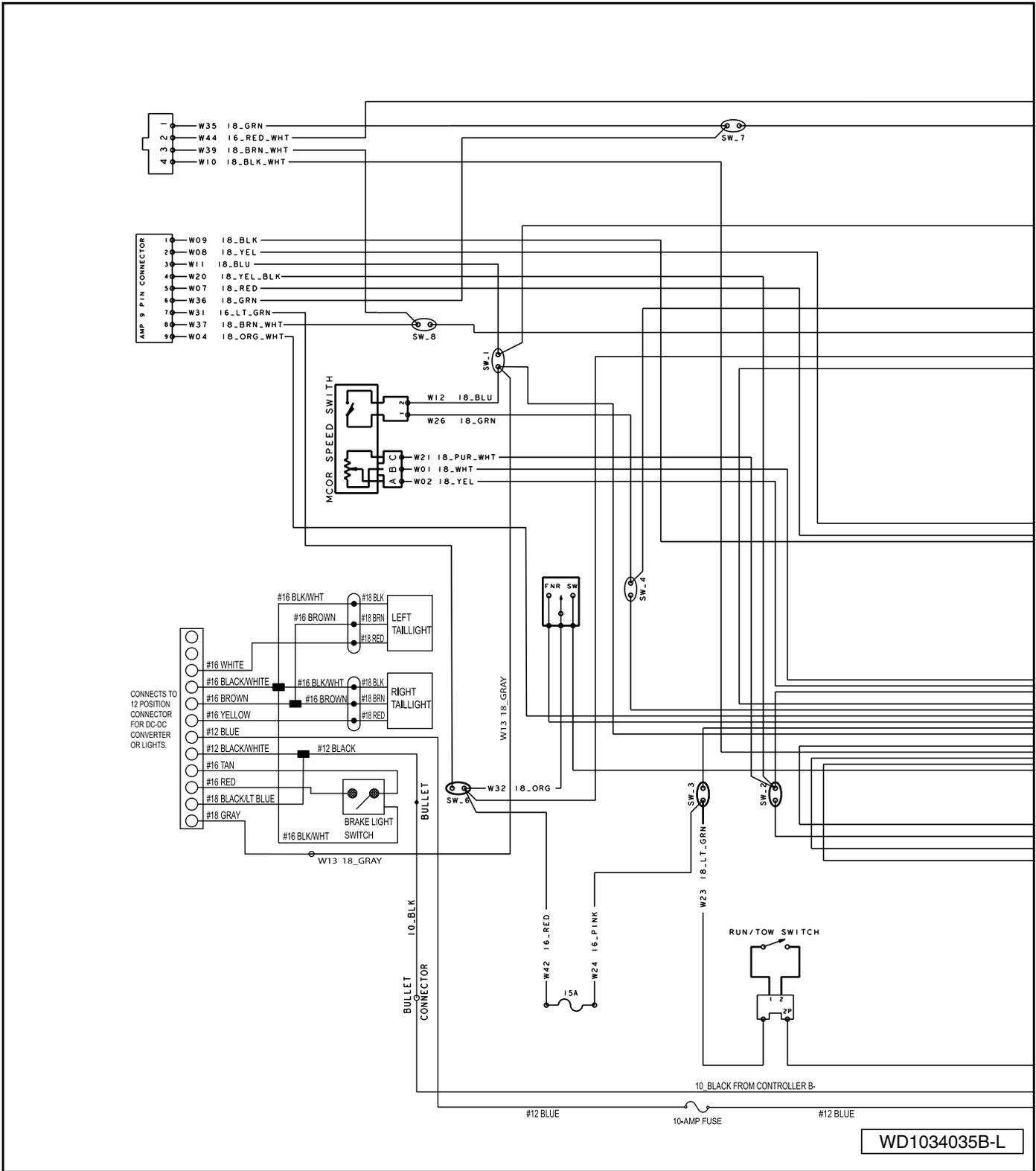
Figure 14-4 Wiring Diagram – Excel System with MCOR
