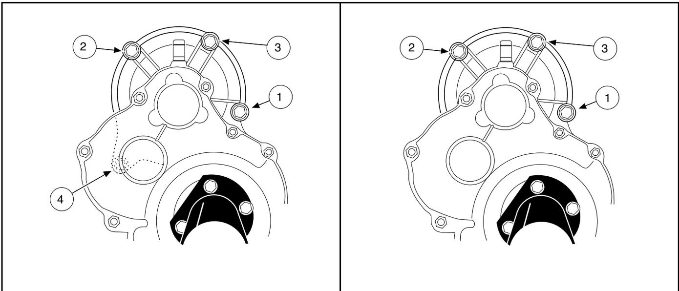
746 **Figure 20-24 EJ4-4001 Motor Mounting Bolts and Tightening Sequence**
