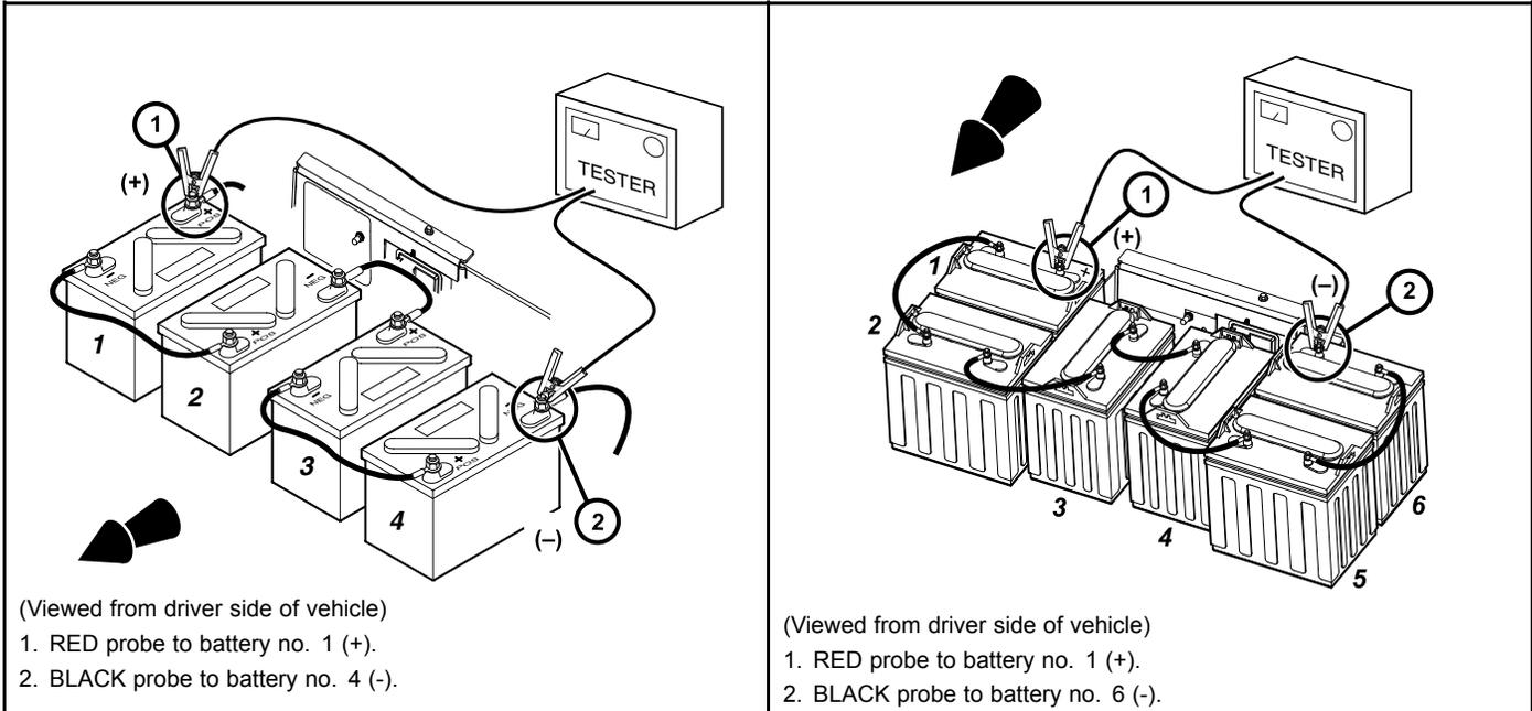
**Figure 14-10 Battery Discharge Test – Style B Battery Configuration**
