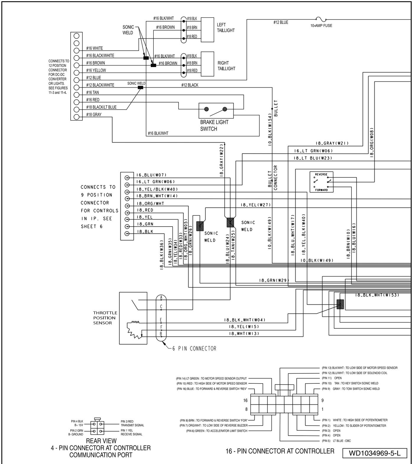
Figure 11-1 Wiring Diagram – IQ System with TPS
