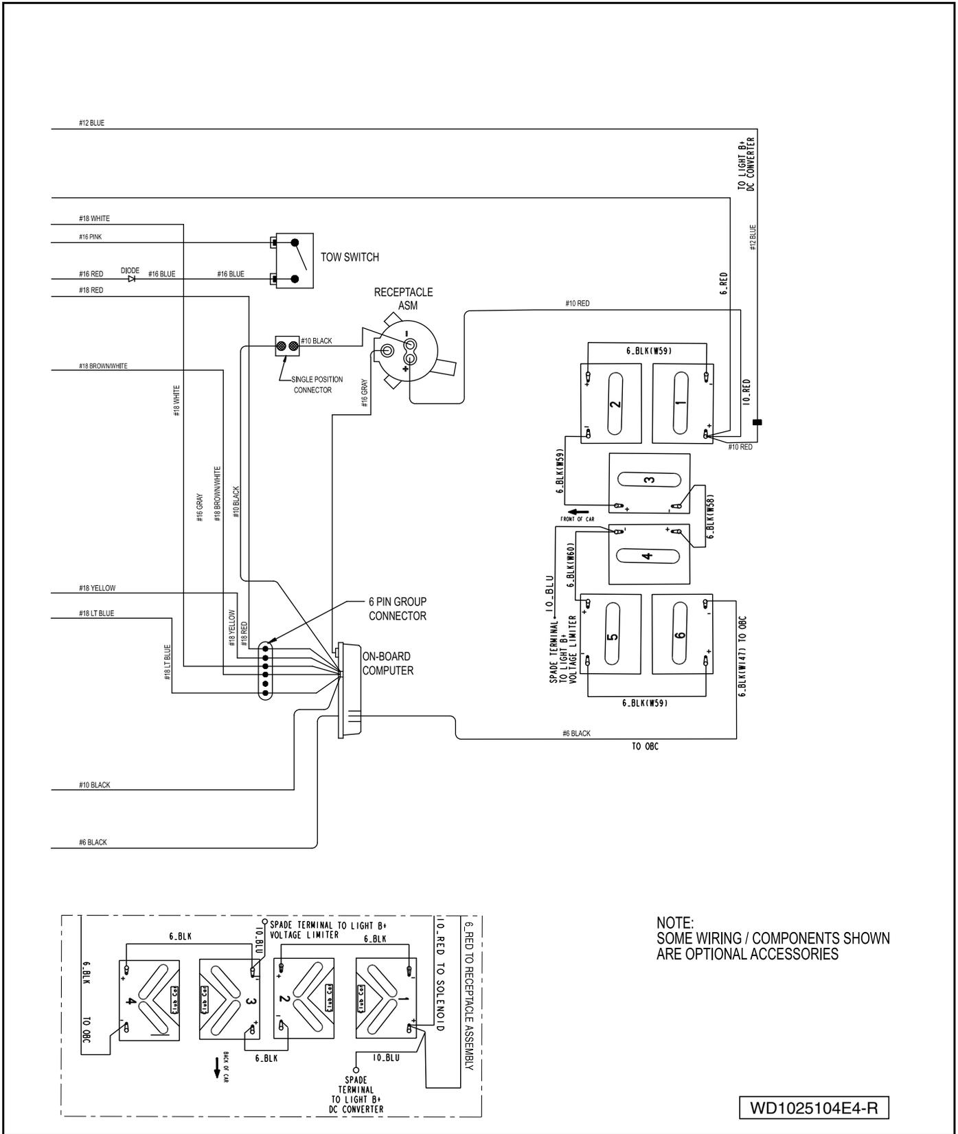
Figure 12-2 Wiring Diagram – IQ System with MCOR (Continued)
