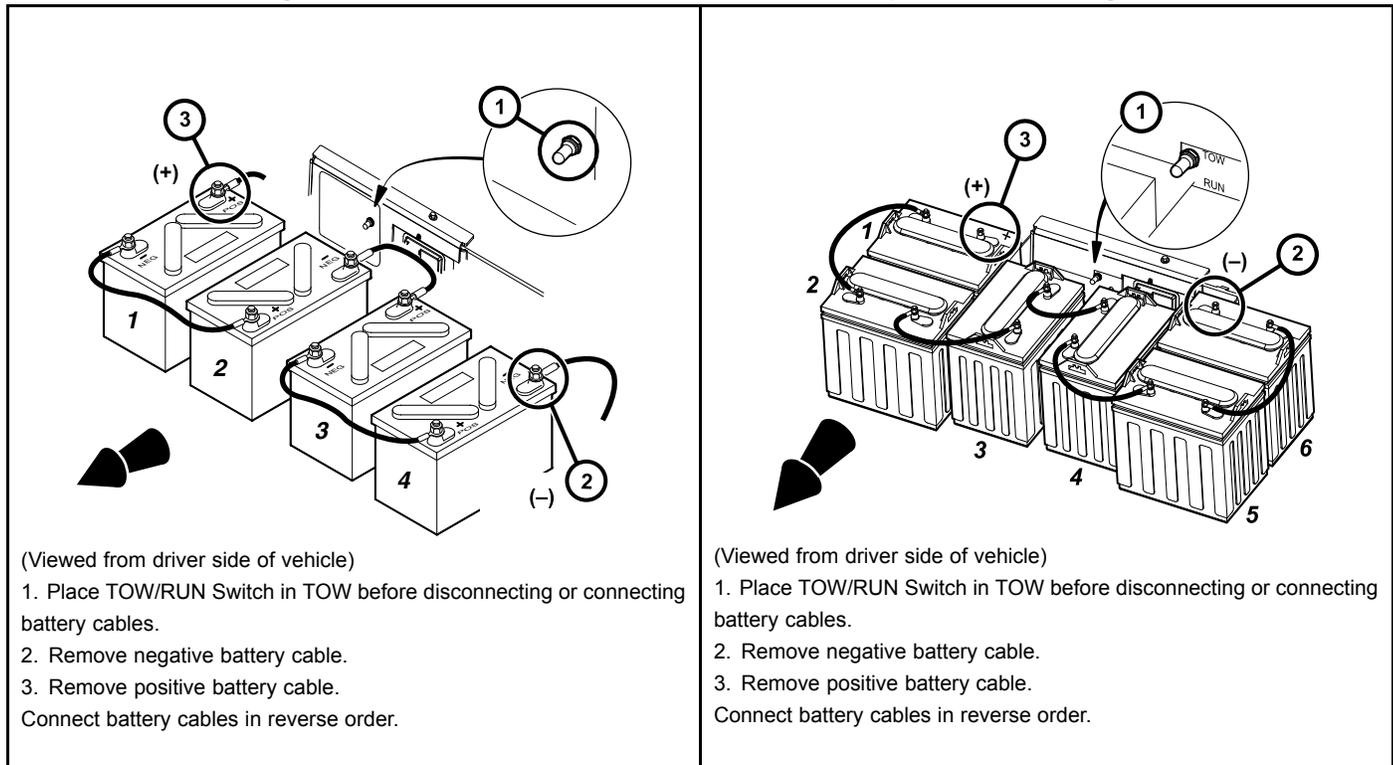
422 **Figure 1-1 Battery Cable Removal – 4x12-Volt Battery Configuration**
