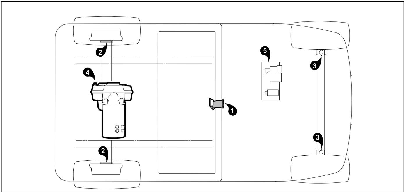
Figure 10-3 Vehicle Lubrication Points
