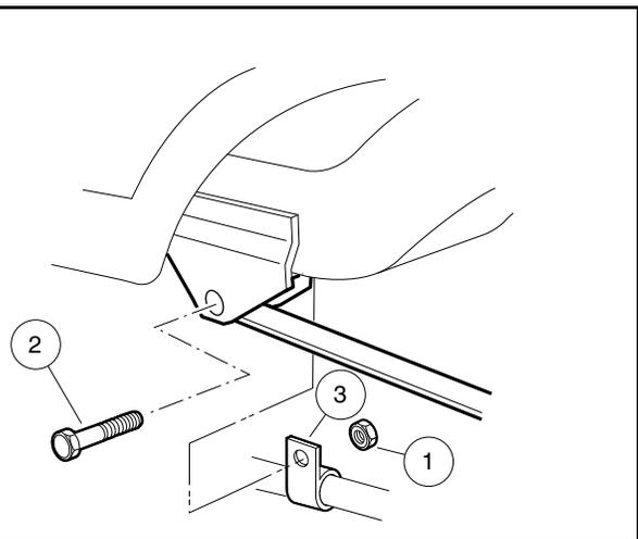
**Figure 6-22 Brake Cable Mounting Tab****BRAKE CABLE INSTALLATION****⚠ WARNING**
