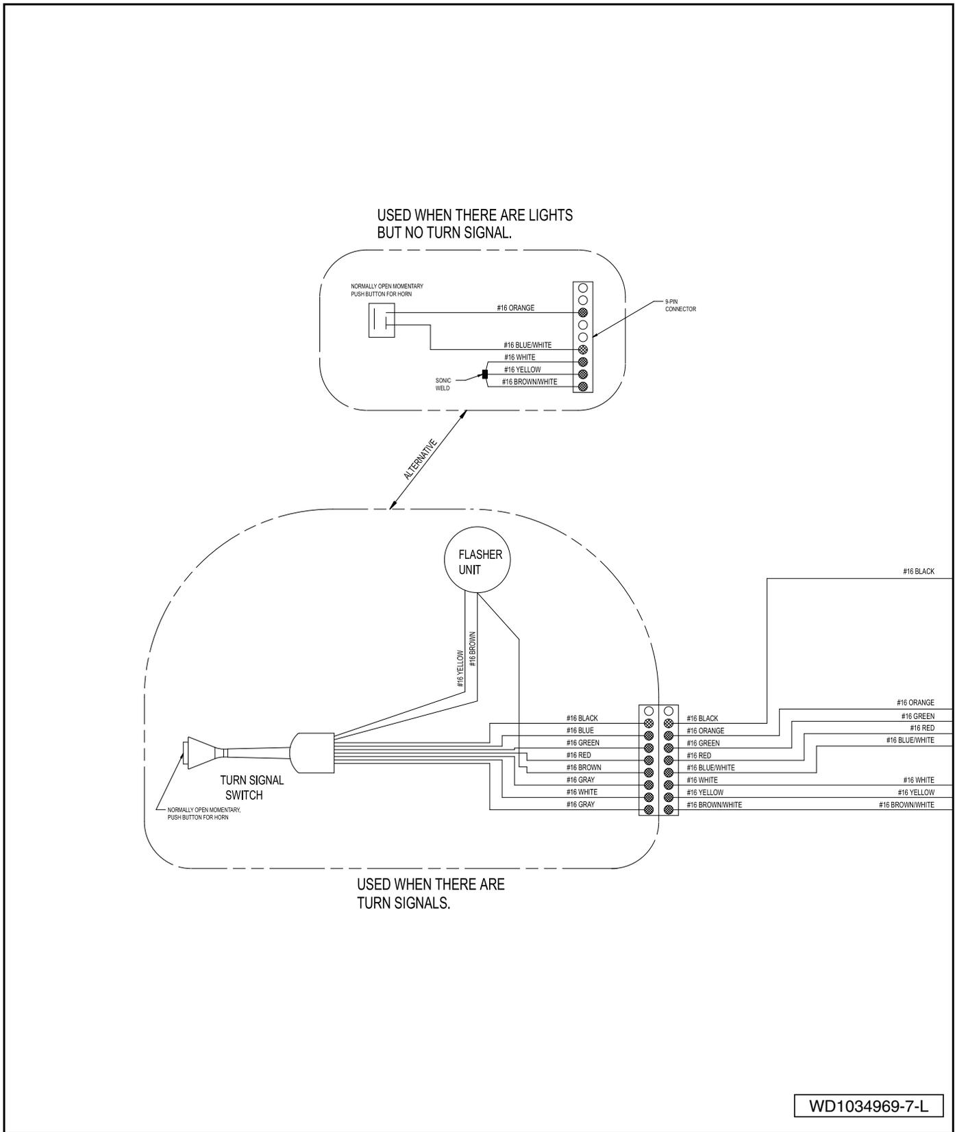
Figure 13-2 Precedent Electric Vehicle Accessory Wiring Diagram
