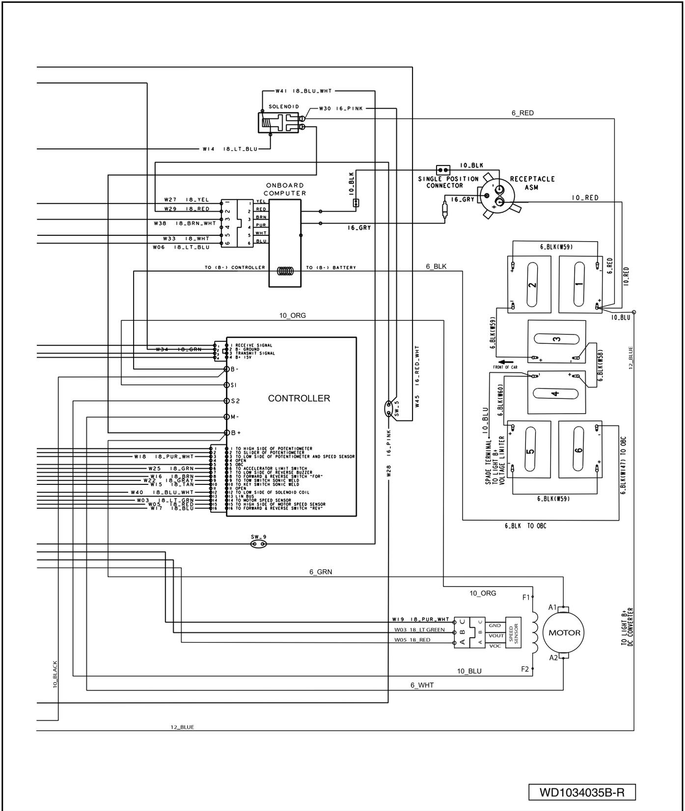
Figure 14-5 Wiring Diagram – Excel System with MCOR (Continued)
