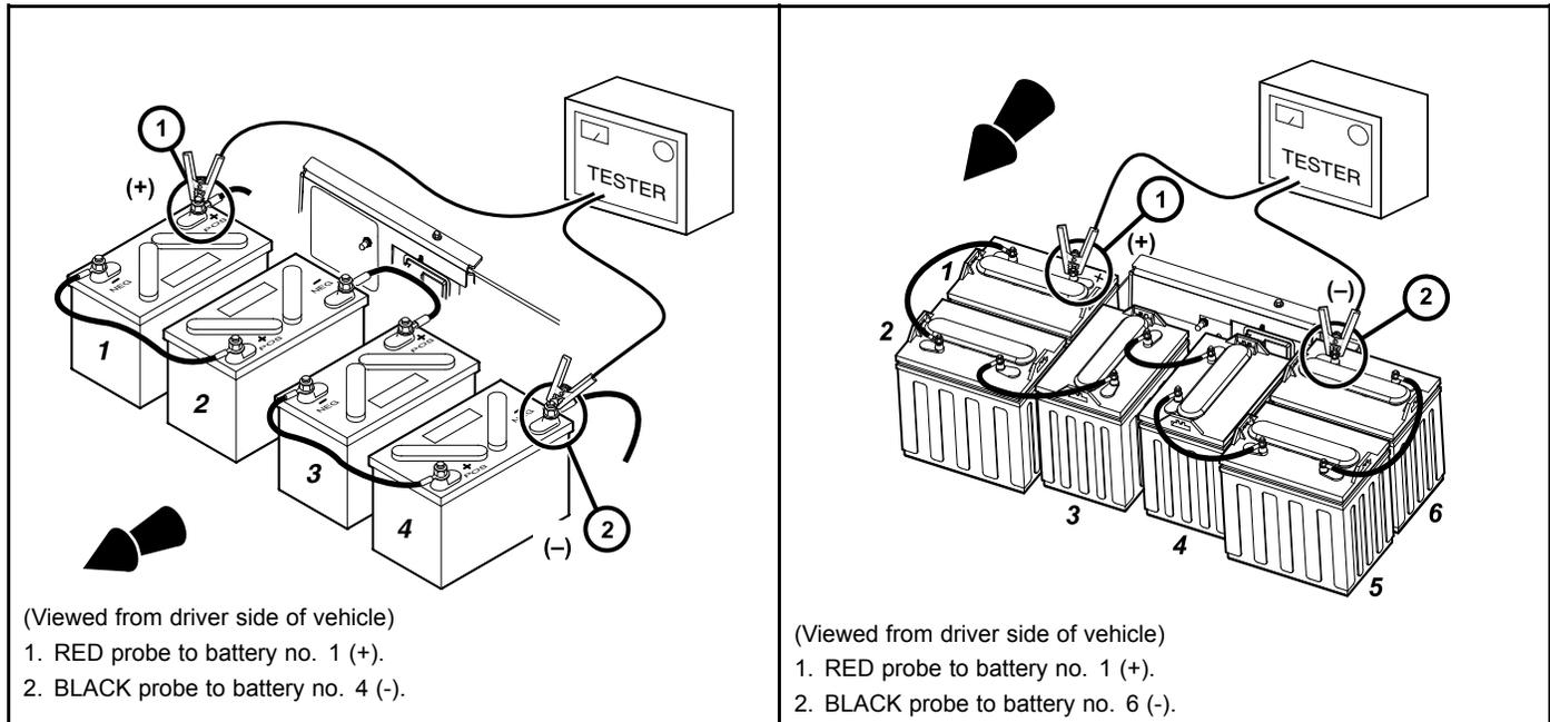
**Figure 13-10 Battery Discharge Test – 4 x 12 Volt Battery Configuration**
