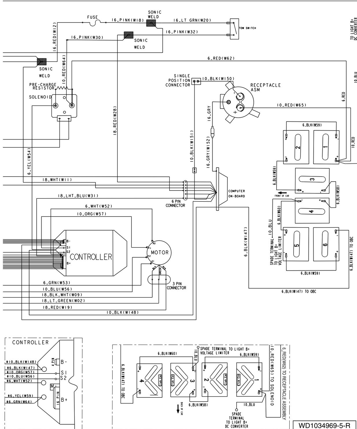
Figure 11-2 Wiring Diagram – IQ System with TPS (Continued)
