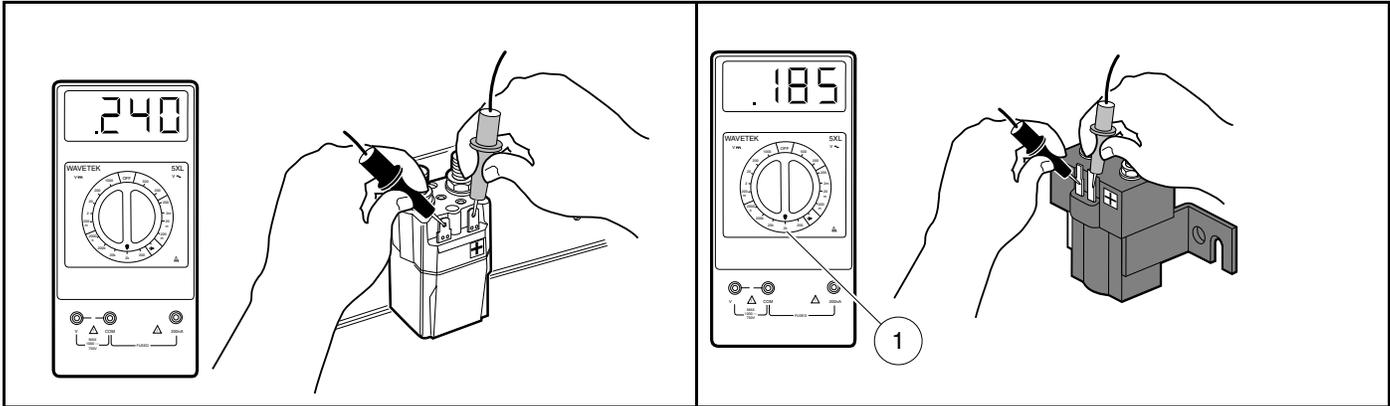
**Figure 14-8 Activating Coil Test – Factory-installed Solenoid**
