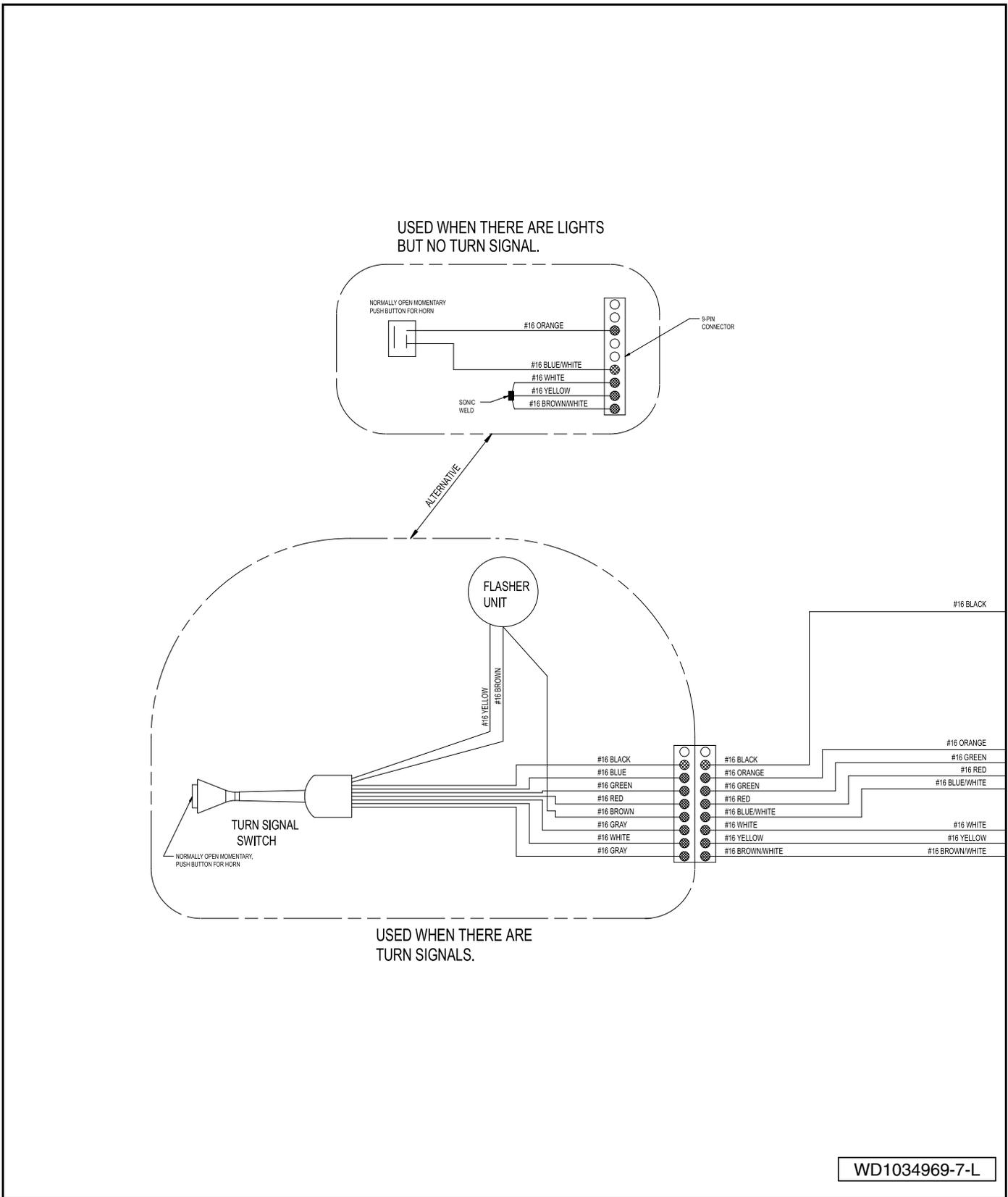
Figure 11-3 Precedent Electric Vehicle Accessory Wiring Diagram
