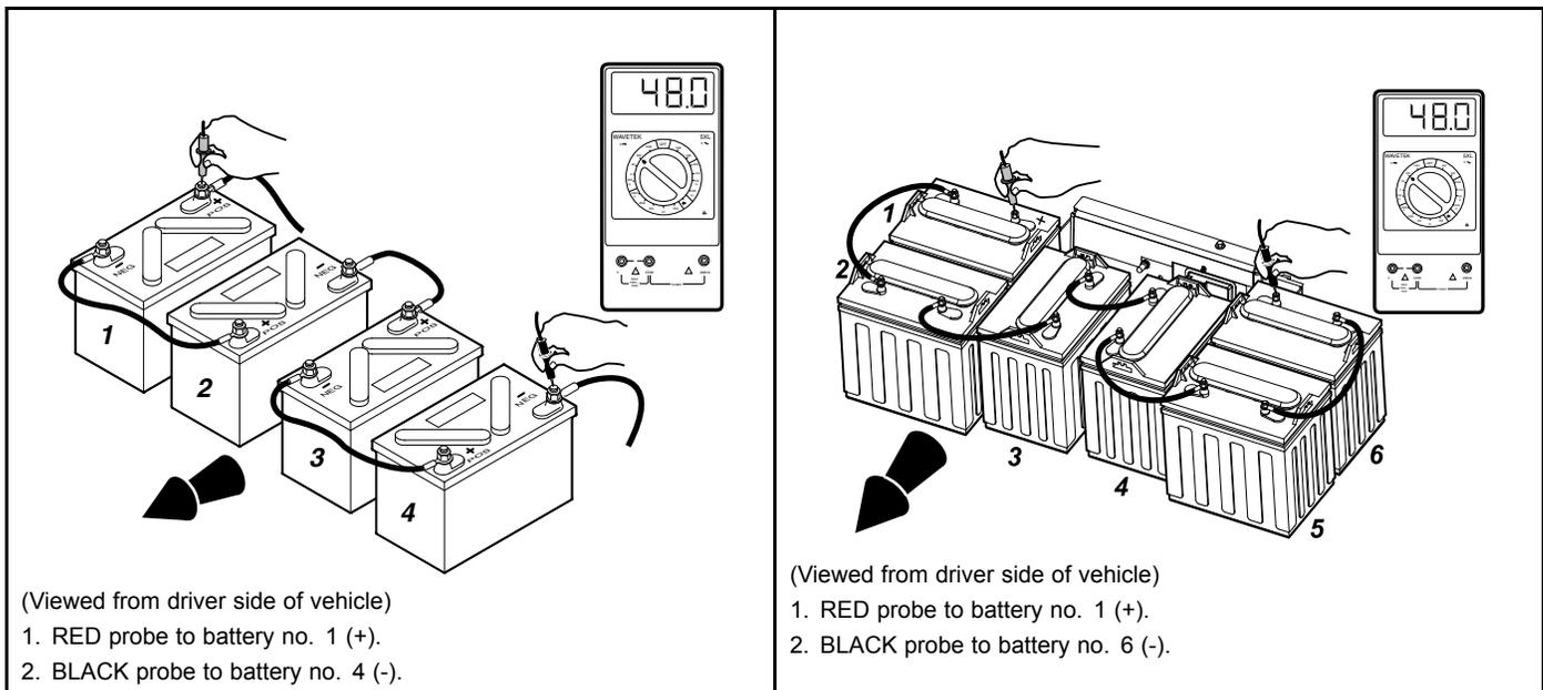
**Figure 11-6 Battery Voltage Test – 4 x 12 Volt Battery Configuration**
