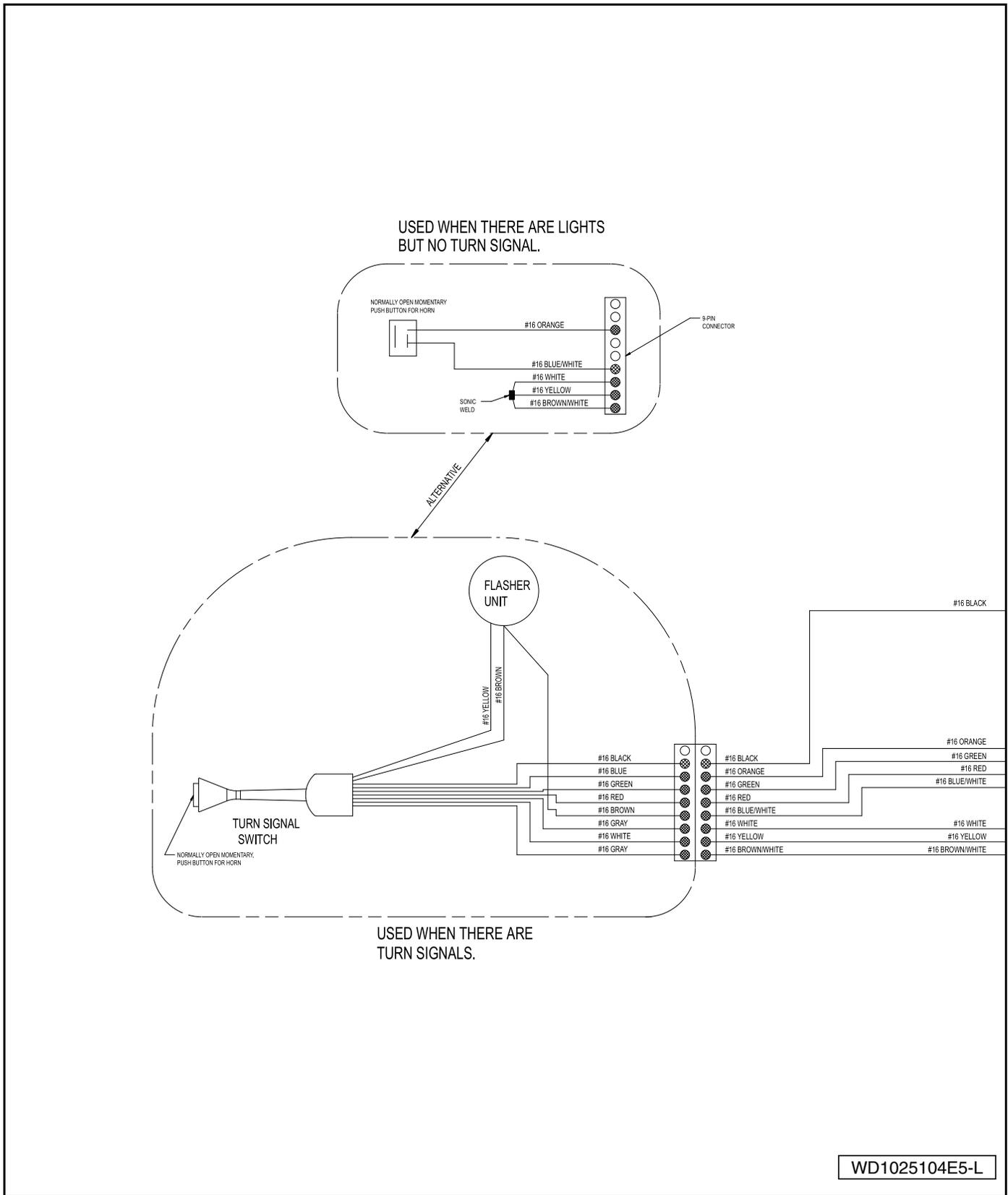
Figure 14-2 Precedent Electric Vehicle Accessory Wiring Diagram
